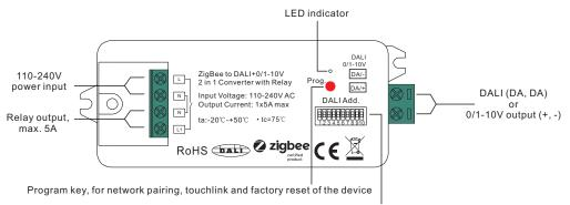
Dip switches to select DALI or 0/1-10V output, DALI DT6 or DT8 color type, DALI address or group control mode, DALI address to be controlled, DALI group to be controlled
